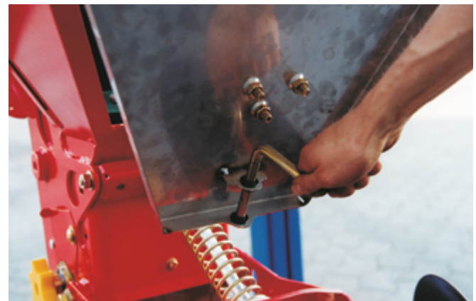
The seed bowl can quickly be emptied, with the opening of the stainless-steel lid.
