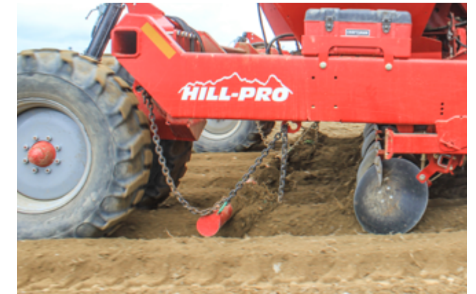
Different shanks are available to loosen the soil to improve tuber growth. They can be positioned in front of, or behind the row unit, and in the rear of the planter. To determine plant emergence, a drag pipe is available to set the hill depth.
