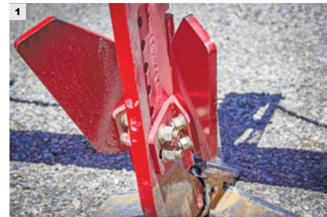
(1) Adjustable wings help funnel more soil onto the row. (2) Hydraulic rock protection with hydraulic reset system. Upon activation the shank is raised and then lowered with controlled hydraulic pressure, eliminating stress to the frame.
