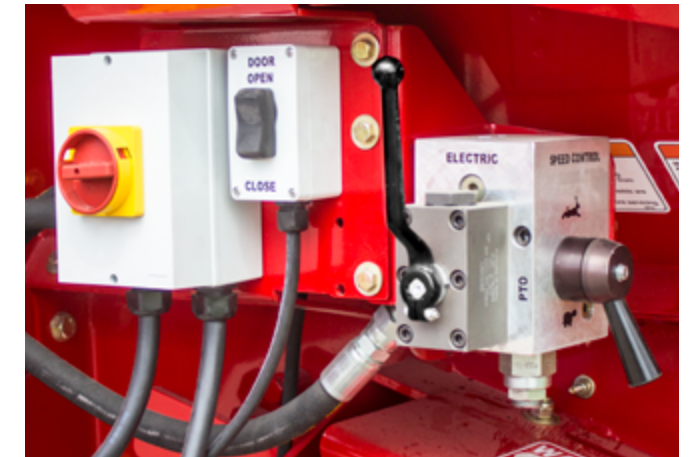
The function controls are centrally located and easily accessible. A selector valve chooses between electric or PTO drive and with a lever, the belt speed is set.
