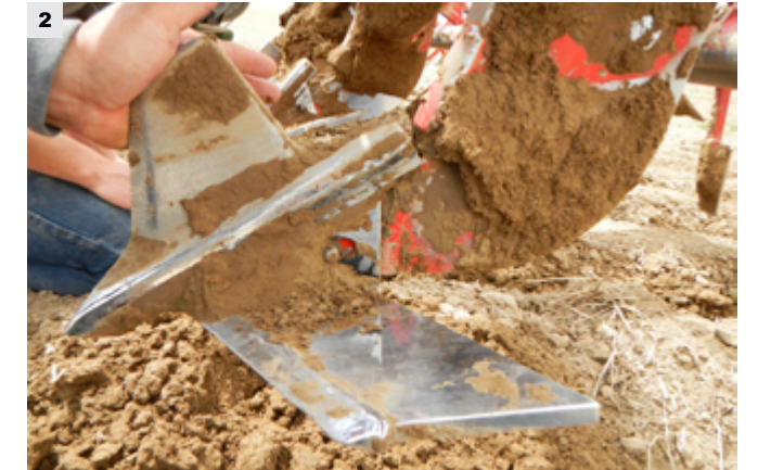
(1) Compared to other systems (shown in black), the shank is closer to the tractor, reducing side shift and the possibility of disturbing the fragile hair roots of the planted seed piece. (2) The wide ripper shanks loosen and aerate the soil.
