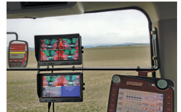
A video-system is available, to track the planting process and monitor key functions.
