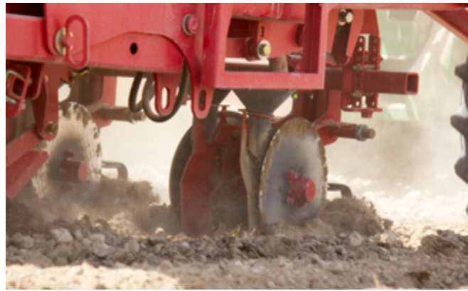
The dry-fertilizer option is available to efficiently place the fertilizer at the correct rate and depth for optimal plant growth. The fertilizer is applied in two bands, next to the seed piece, for a consistent growth pattern.
