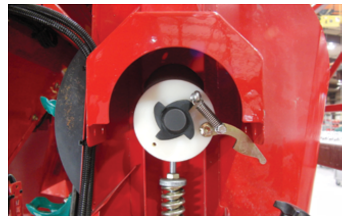
For spraying tracks or on wedge-shaped fields, the planting elements can be individually switched off mechanically.
