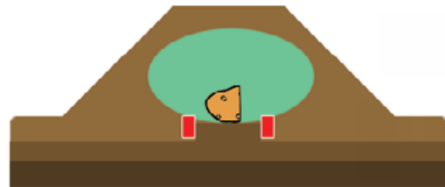
The dry-fertilizer option is available to efficiently place the fertilizer at the correct rate and depth for optimal plant growth. The fertilizer is applied in two bands, next to the seed piece, for a consistent growth pattern.
