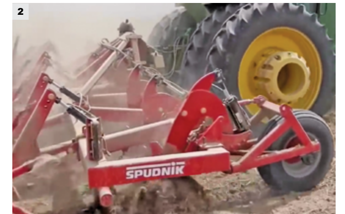
(1) Adjustable wings help funnel more soil onto the row. (2) Hydraulic rock protection with hydraulic reset system. Upon activation the shank is raised and then lowered with controlled hydraulic pressure, eliminating stress to the frame.
