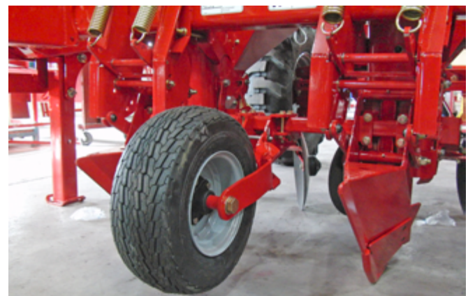
The gage wheels are available in two sizes, for individual depth control of two rows.
