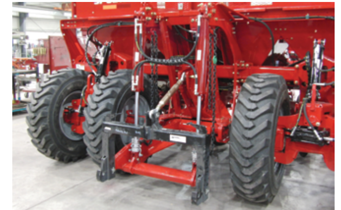
To reduce the number of passes in the field, a three-point hitch is available to mount additional implements.
