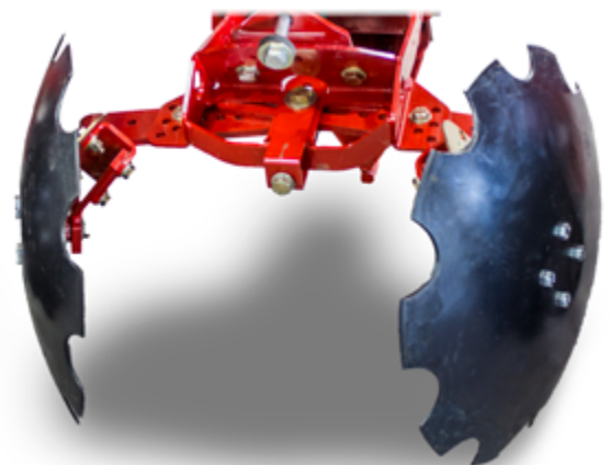
The spring-loaded discs cover the potato with dirt and form a preliminary hill. The external hub with bearings are reliable, and maintenance free. Diameters of 18" (46 cm) or 20" (50 cm) are available in a straight or serrated disc.
