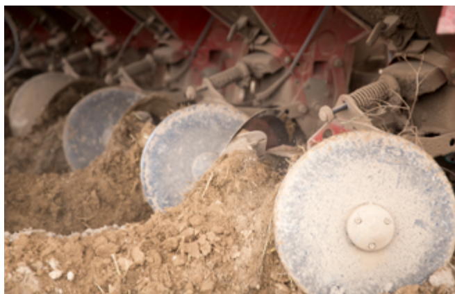
The spring-loaded discs cover the potato with dirt and form a preliminary hill. The external hub with bearings are reliable, and maintenance free. Diameters of 18" (46 cm) or 20" (50 cm) are available in a straight or serrated disc.
