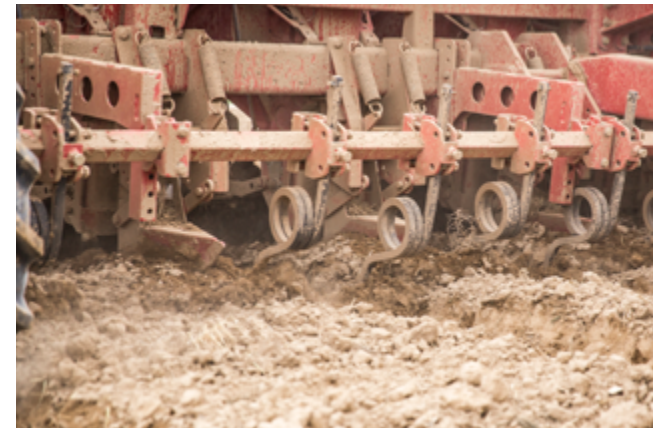
Different shanks are available to loosen the soil to improve tuber growth. They can be positioned in front of, or behind the row unit, and in the rear of the planter. To determine plant emergence, a drag pipe is available to set the hill depth.
