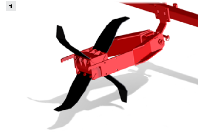
Props eliminate water run off and conserve valuable moisture. The Spudnik prop (1) creates a deep pocket without removing soil from the hill. The Sunco prop (2) creates an angled pocket minimizing vehicle rocking when field working.
