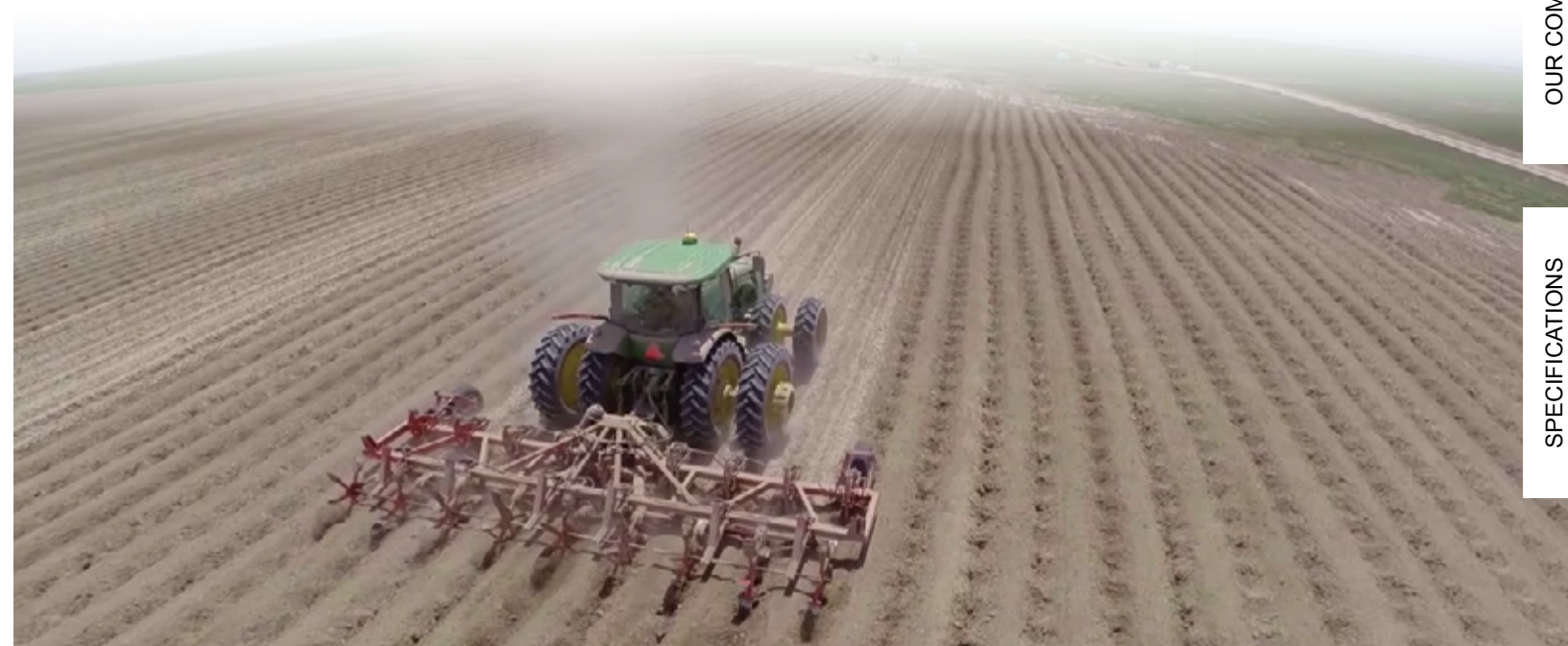
(1) Adjustable wings help funnel more soil onto the row. (2) Hydraulic rock protection with hydraulic reset system. Upon activation the shank is raised and then lowered with controlled hydraulic pressure, eliminating stress to the frame.
