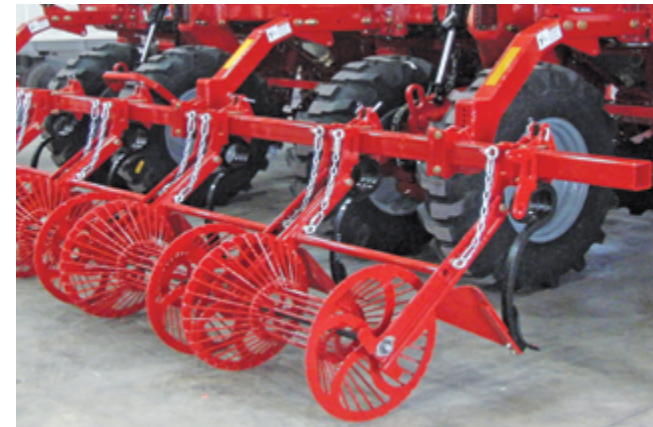
The cage roller improves water absorption in light soils, as well as creating a more stable row, in irrigated fields.
