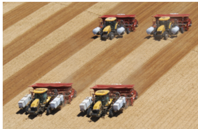
GPS capable planters, with steerable axles, to take advantage of precision farming. For fields with side hills, it is especially important for correct seed and row alignment to reduce green ends on the tubers.
