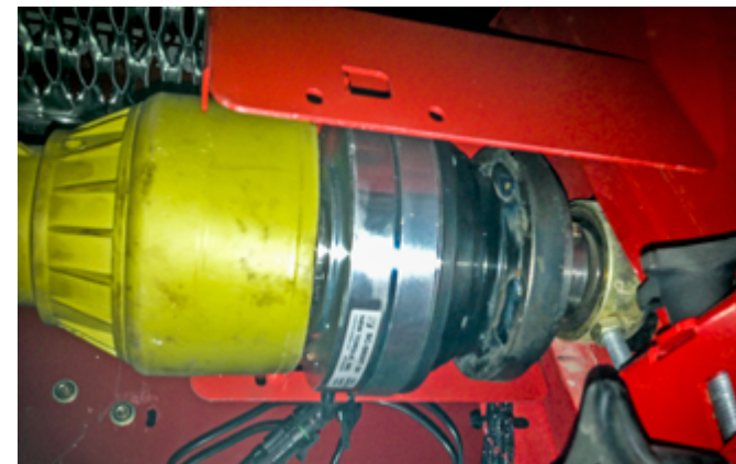
To switch off each row unit independently, for headland management or seed planting, an electric clutch is available.
