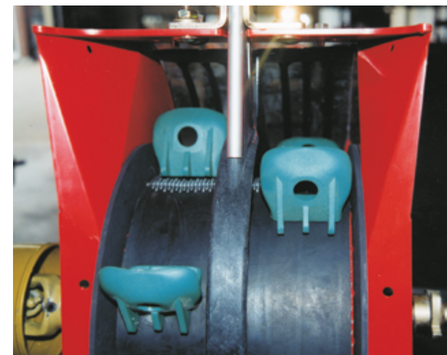
The large funnel-shaped inlet makes it possible to reliably plant a variation of seed sizes.
