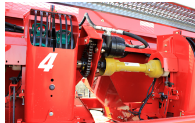
Hydraulically-driven row unit: Independent of ground speed, used for variable seed rating. A mechanical drive is available.
